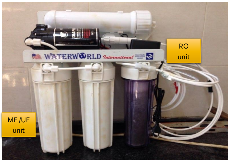
Figure (4.4): Reverse osmosis filter unit
