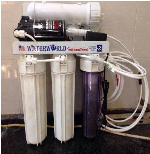
Figure (5.2): MF/UF &RO unit
