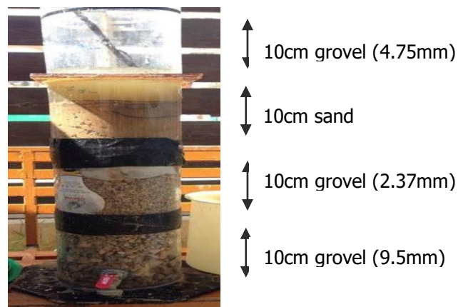
Figure (4.3): Sand filter configuration 'trial2'
